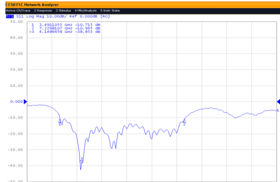
Figure 10: S11 of Fabricated Fractal Antenna
