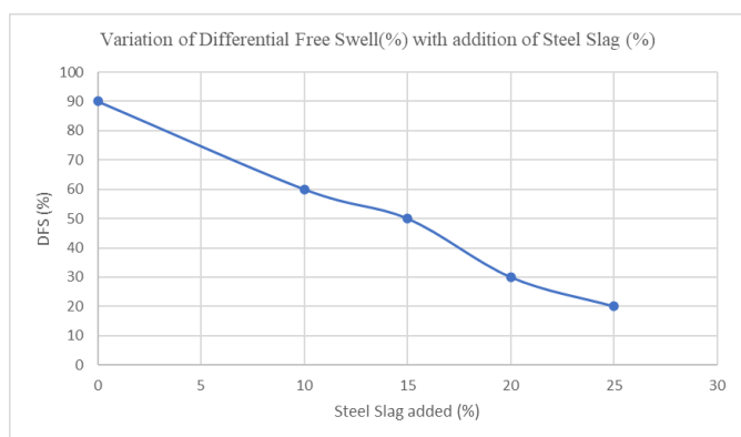
Chart-7: Variation of Differential Free Swell with percentage variation of steel slag (%)
