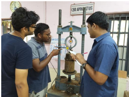
Fig.1: Authors conducting CBR test
