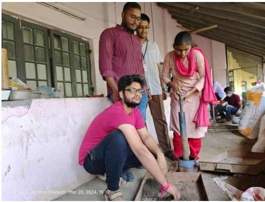
Fig.2: Authors performing Modified Proctor Compaction
