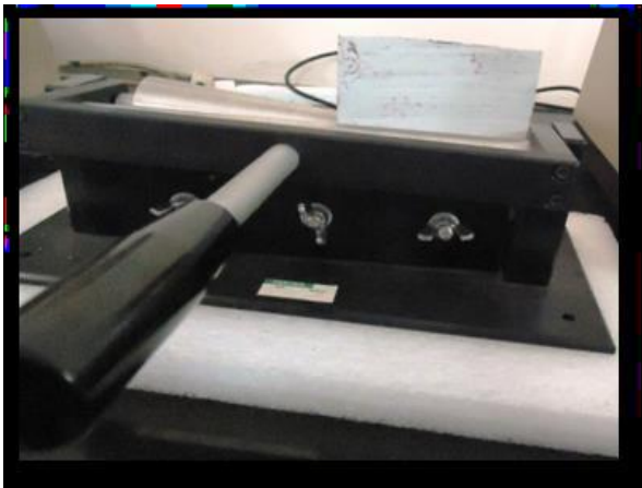
Fig.-4: Conical Mandrel Apparatus
