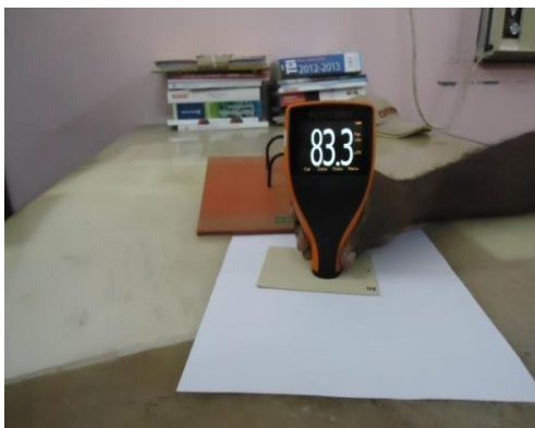
Fig.-2: Measuring coating thickness
