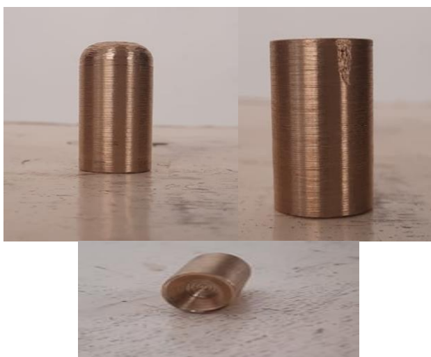
Fig-2: Convex, Flat & Concave Profile Electrode
