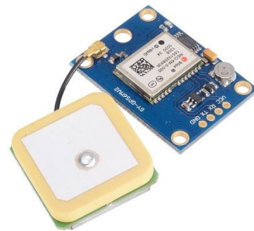
Fig -4: GPS Module with Patch Antenna
