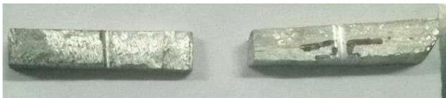
Fig 6.3 Toughness sample of 2.5 % of Alumina in aluminum
