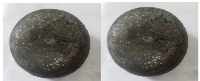
Figure 5.1 Sample of aluminium + Al 2 O 3 2.5 and 5% Alumina in Aluminium
