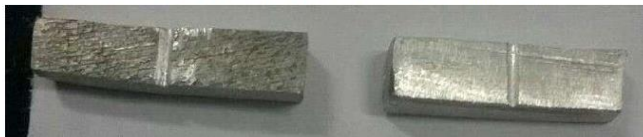
Fig 6.4 Toughness sample of 5% of Alumina in aluminum
