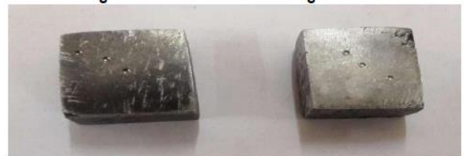
Figure 6.8 MMC sample after pockmark on Hardness Testing Machine
