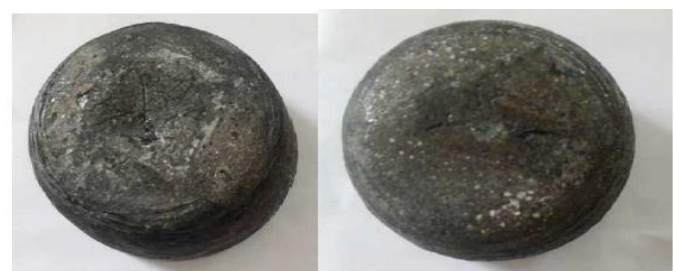
Figure 5.2 Sample of aluminium + Al 2 O 3 7.5 and 10% Alumina in Aluminium
