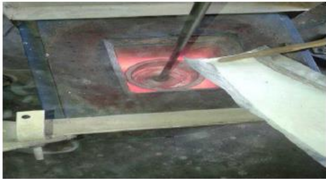
Figure 5.3 Preparation of sample by mechanical stir casting
