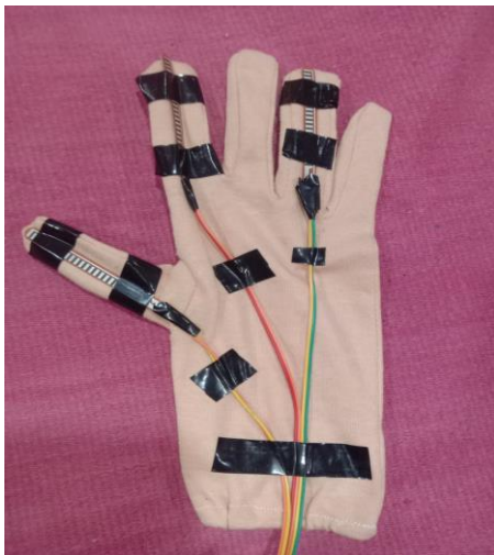
Fig 3.2:: Human hand glove with Flex Sensor
