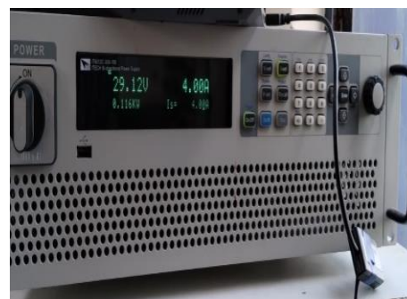
Fig -3 : Bi-directional Power Supply delivering > 100W Power
