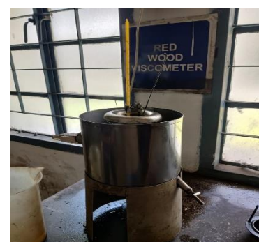
Figure-5: Redwood viscometer test
