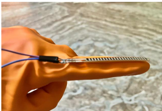
Figure 2 – The Flex Sensor is attached to the glove
