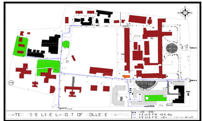
Fig.1 Existing Pipe Distribution Network
