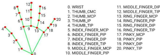
Fig. 1 – Localized Hand Landmarks by MediaPipe
