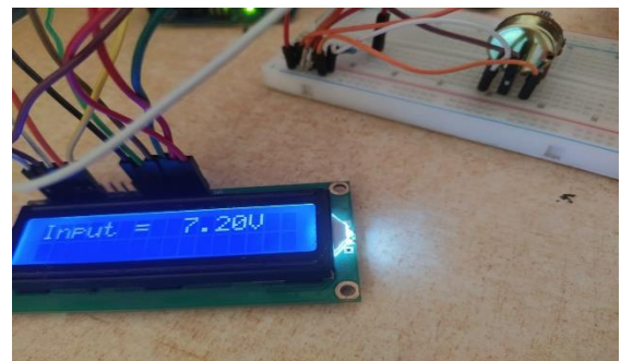
Fig 5 Excess Voltage Displayed on LCD Screen
