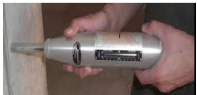
Fig-2: Rebound Hammer
