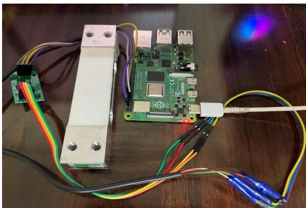
Fig 5: HX711 and weighing module connection with raspberry
