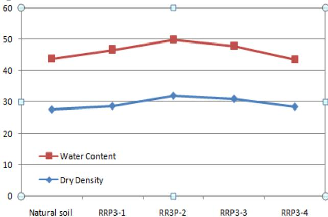
Fig. 2 Proctor compaction Test on natural soil & RRP3 samples
