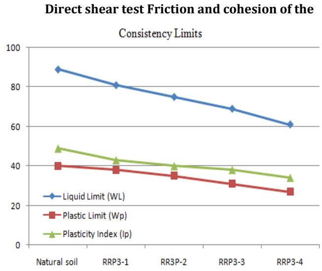
Fig. 1 Atterberg's limits Test on natural soil & RRP3 samples
