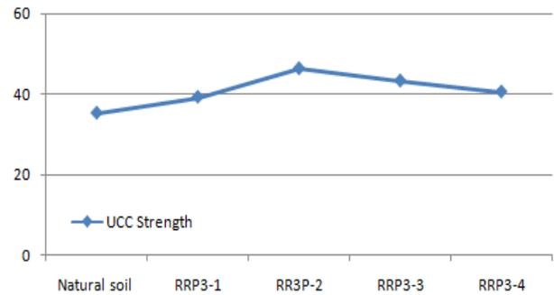
Fig. 3 Unconfined Compression Test on natural soil & RRP3 samples
