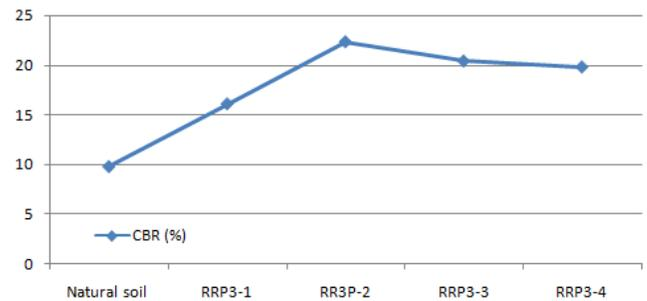
Fig. 4 California Bearing Ratio Test on natural soil & RRP3 samples
