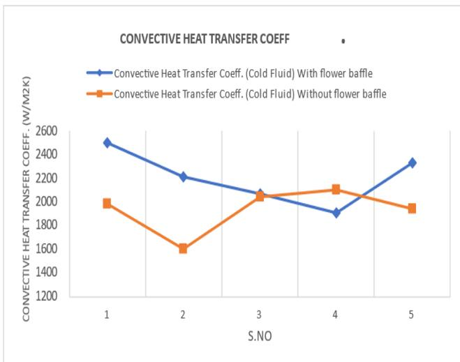
Fig. 5: Graph of Convective heat transfer coefficient in cold fluid.
