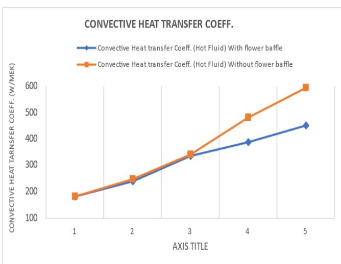
Fig. 6: Graph of Convective heat transfer coefficient in hot fluid
