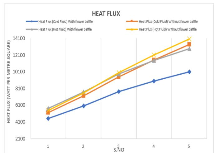
Fig. 4: Graph of heat flux in shell and tube heat exchanger.
