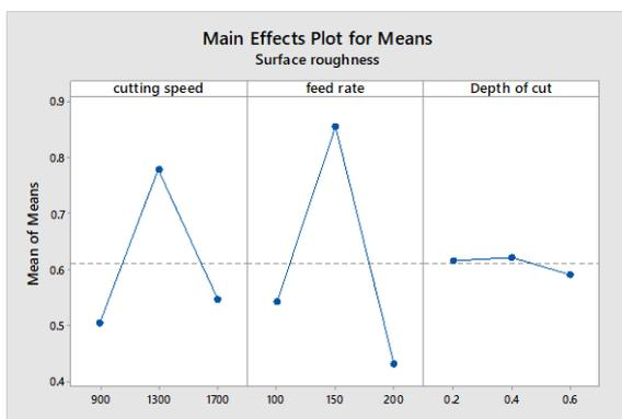
Figure 6 Effect of individual process variables on surface roughness
