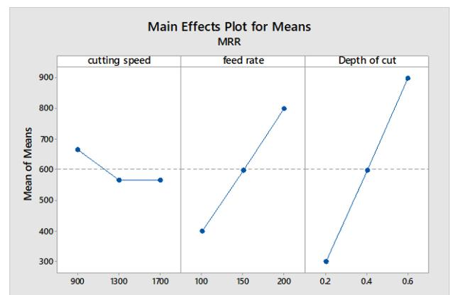
Figure 8 Effect of individual process variables on MRR
