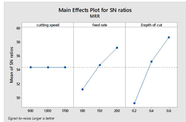
Figure 7 Mean S/N ratio of MRR
