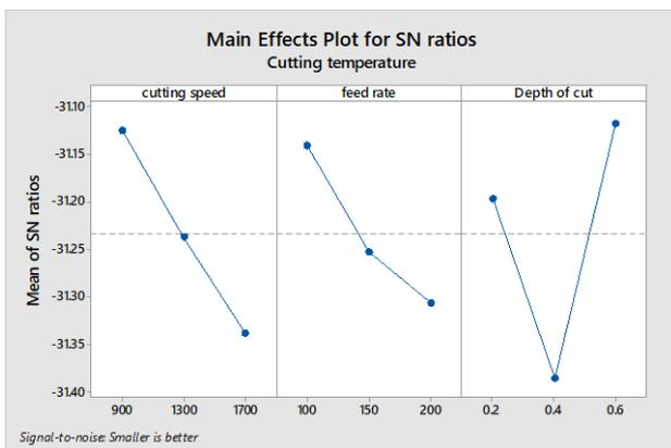
Figure 3 Mean S/N ratio of cutting temperature
