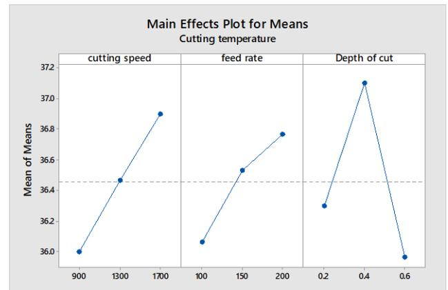
Figure 4 Effect of individual process variables on cutting temperature
