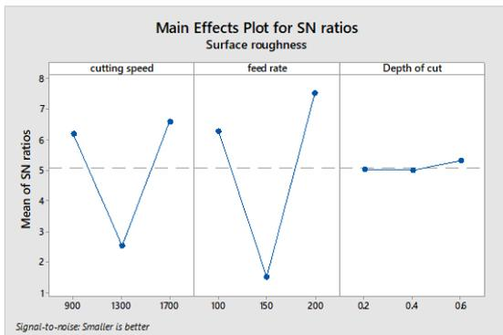
Figure 5 Mean S/N ratio of surface roughness
