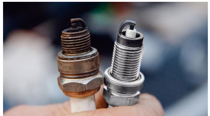
Fig 3: Spark plug failure
