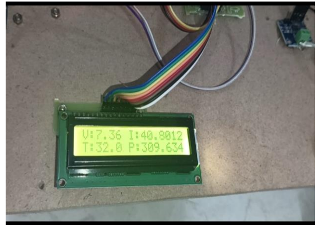
Fig.6: Battery Management Using DTH11, Current Sensor, Potentiometer.
