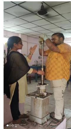
Preparation Of Bituminous Mix Mould
