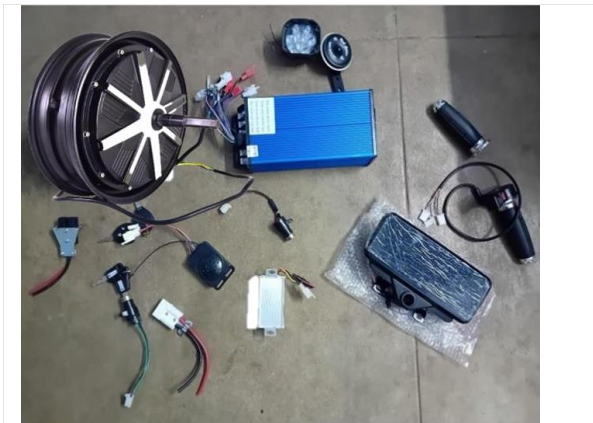
(a) Full kit of electric vehicle conversion
