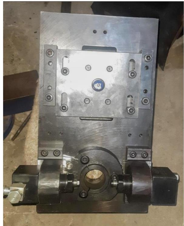
Fig -4: Finish fixture without Component
