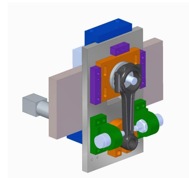
Fig -3: Finish Boring Fixture
