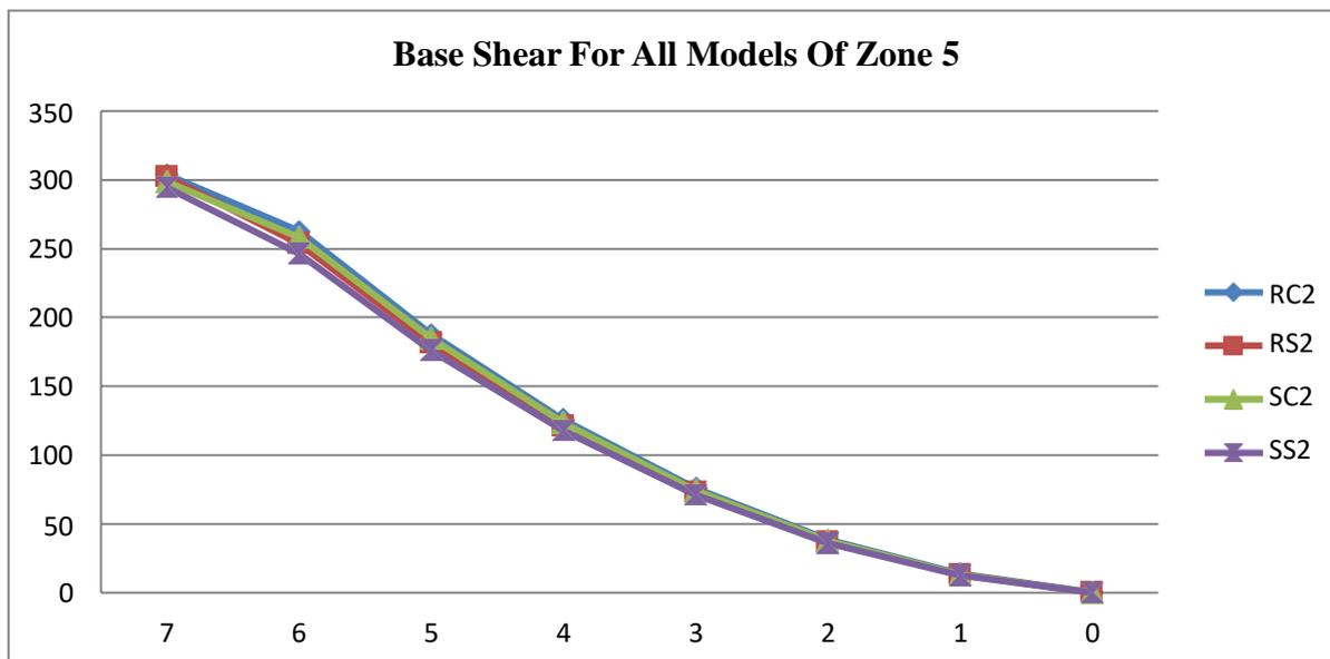
Fig. 5.1.10 Comparison of Base Shear for all models of zone 5
