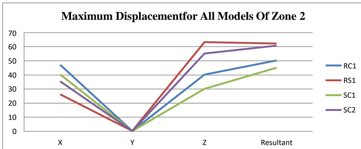
Fig. 5.1.3 Comparison of Maximum Displacement for all models of zone 2
