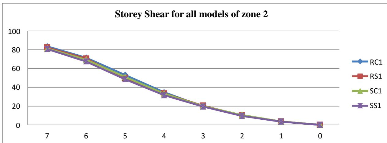
Fig. 5.1.5 Comparison of Storey Shear for all models of zone 2
