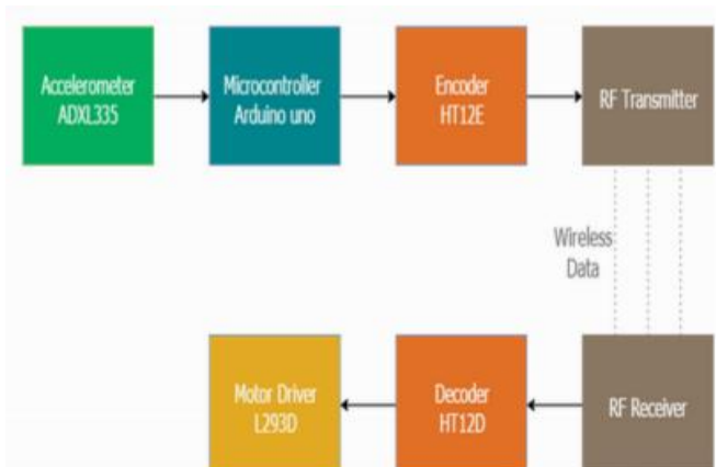
Figure 1 Hand Gestured Controlled Car circuit layout
