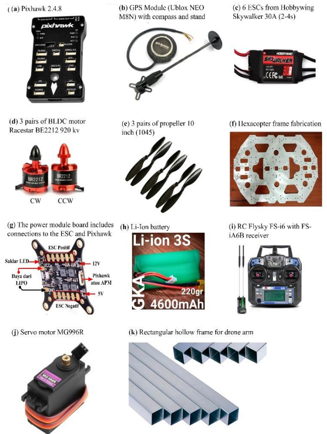
Fig. 2.1 Selection of main components for developing a hexacopter drone that is used for delivering goods
