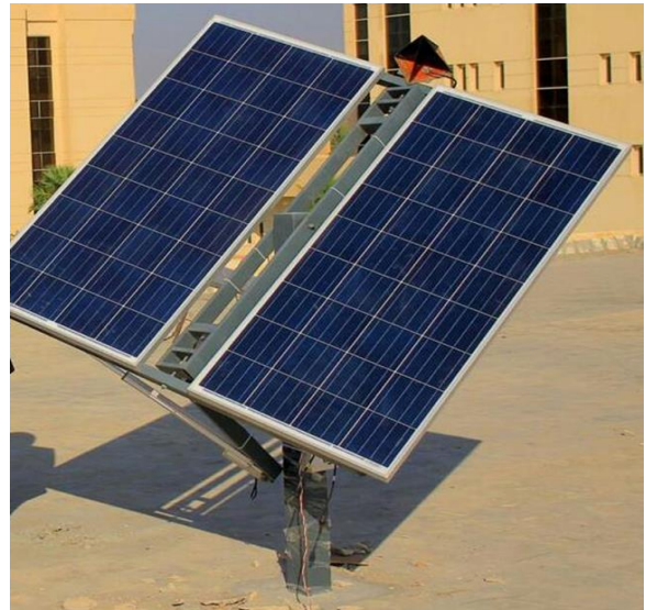
Figure 8. Two PV panel (2*150 watts)
