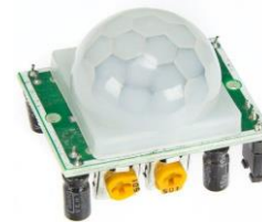
Fig-5: PIR Motion Sensor
