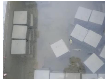
Fig. 15 Curing of Concrete cube
