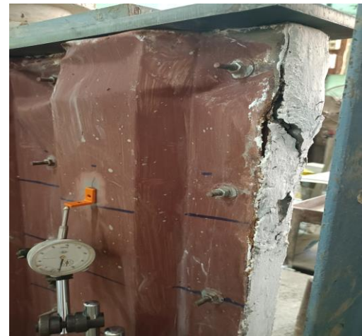
Fig. 6: Crippling of sheet and Diagonal Compression Shear Failure
