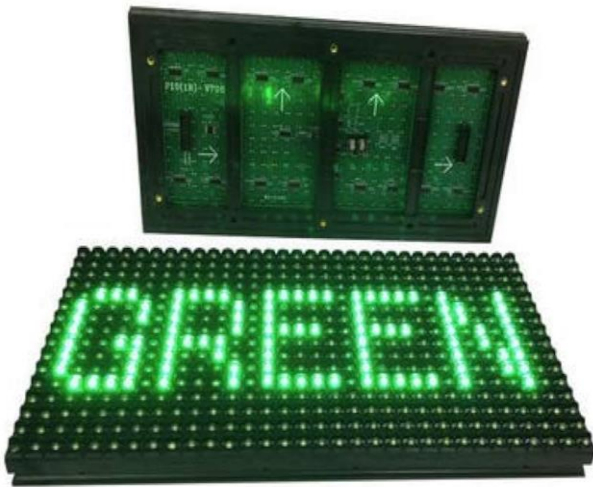
Figure-5: P10 single colour LED
