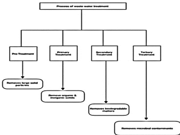
Figure 3. Process of Wastewater Treatment
