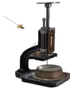
Figure -6: Initial Setting Time - Vicat apparatus with needle.
