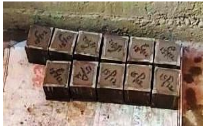
Figure -3: Sample Preparation – Compressive Strength Test
