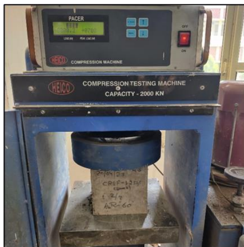
Fig-3: Compression Strength test setup
