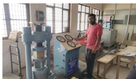
Fig.11 Compression test on concrete blocks
