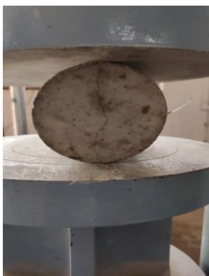
Fig 4.3 Split tensile strength test
