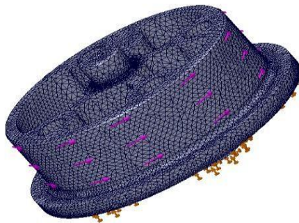
Figure -6: a) Applied Boundary Condition and Torque on old design Hub Idle Gear b) Applied Boundary condition and Torque on old design Hub Idle Gear
