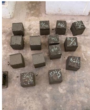
Fig. 2.6 Drying and Demoulding of cubes.
