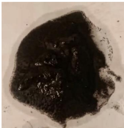
Fig -9: RHA after HCl reflux
