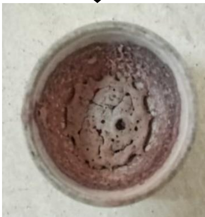
Fig -10: Residue burnt in muffle furnace
