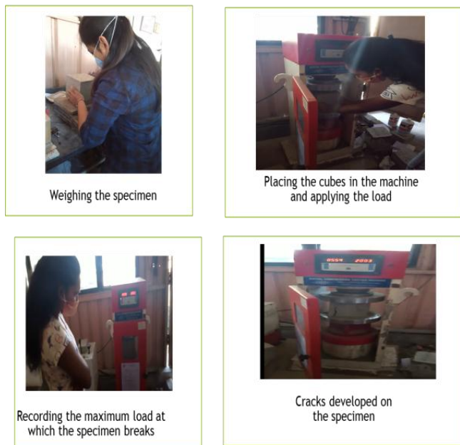
Fig -4: Compressive strength testing
