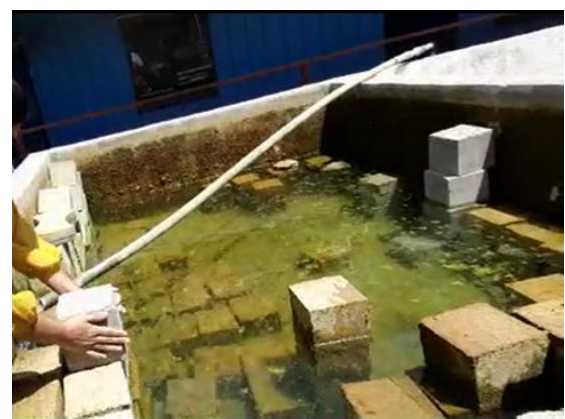
Fig -3: Curing of cubes
