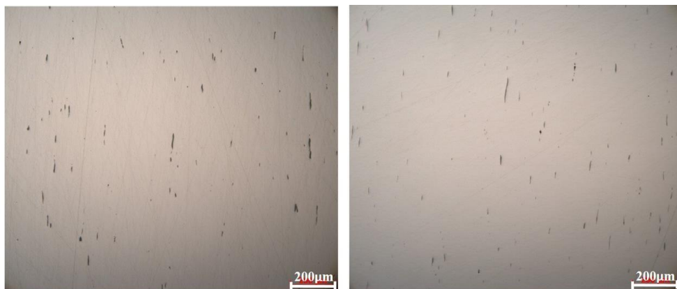
Fig-3: Optical image of the inclusion in new bolt(a) and failed bolt (b).
