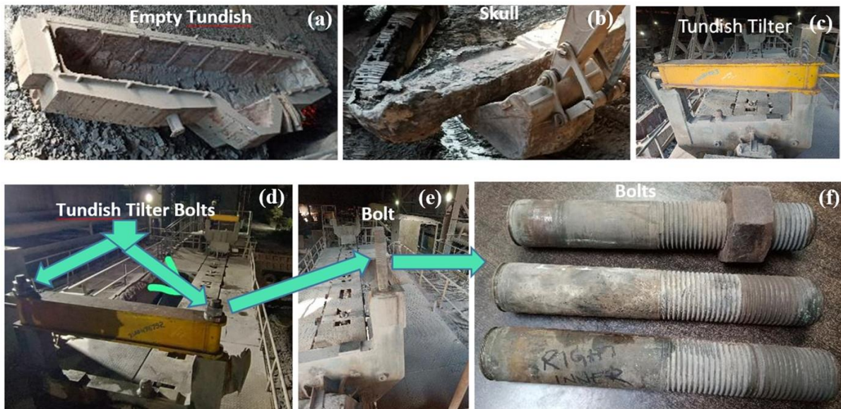
Fig-1: (a) Empty Tundish (b) Skull (c) Tundish Tilter (d)-(f) Tundish Tilter Bolts.
