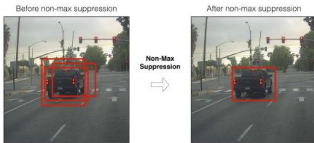
Fig. 7. The YOLO technique's non-max reduction function only retains best-fit bounds. [24]
