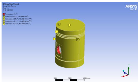
Fig 8: Thermal analysis of piston
