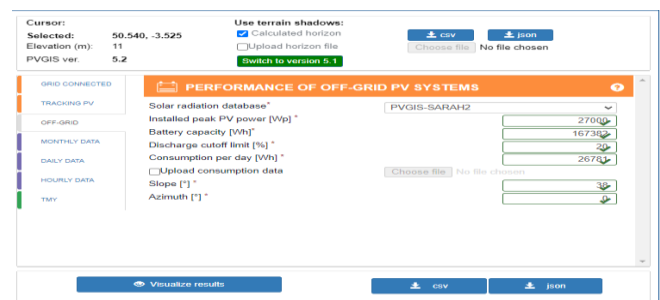
Fig 2: Solar electricity generation using PVGIS tool
