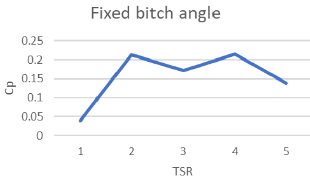
Figure 15: Coefficient of performance of portable wind turbine under normal operation.
