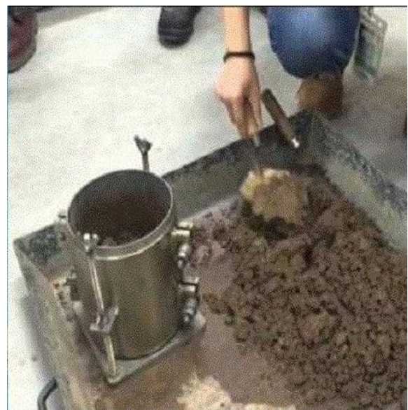
Fig. 5 Sample for observing compaction values of soil
