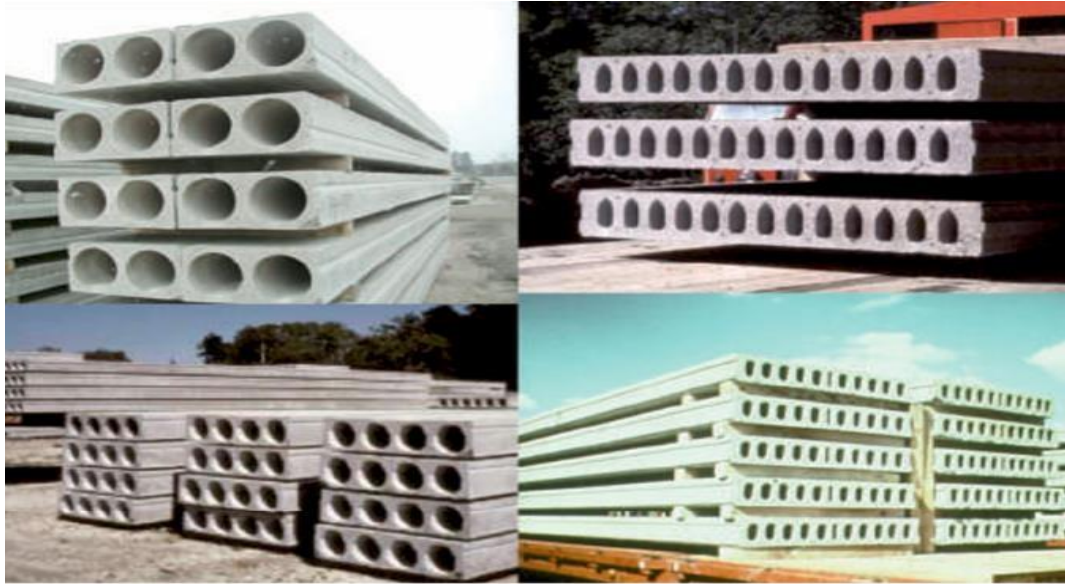
Figure 2: Precast hollow-core slabs stacked at yard and jobsite, PCI, 2017 [2]
