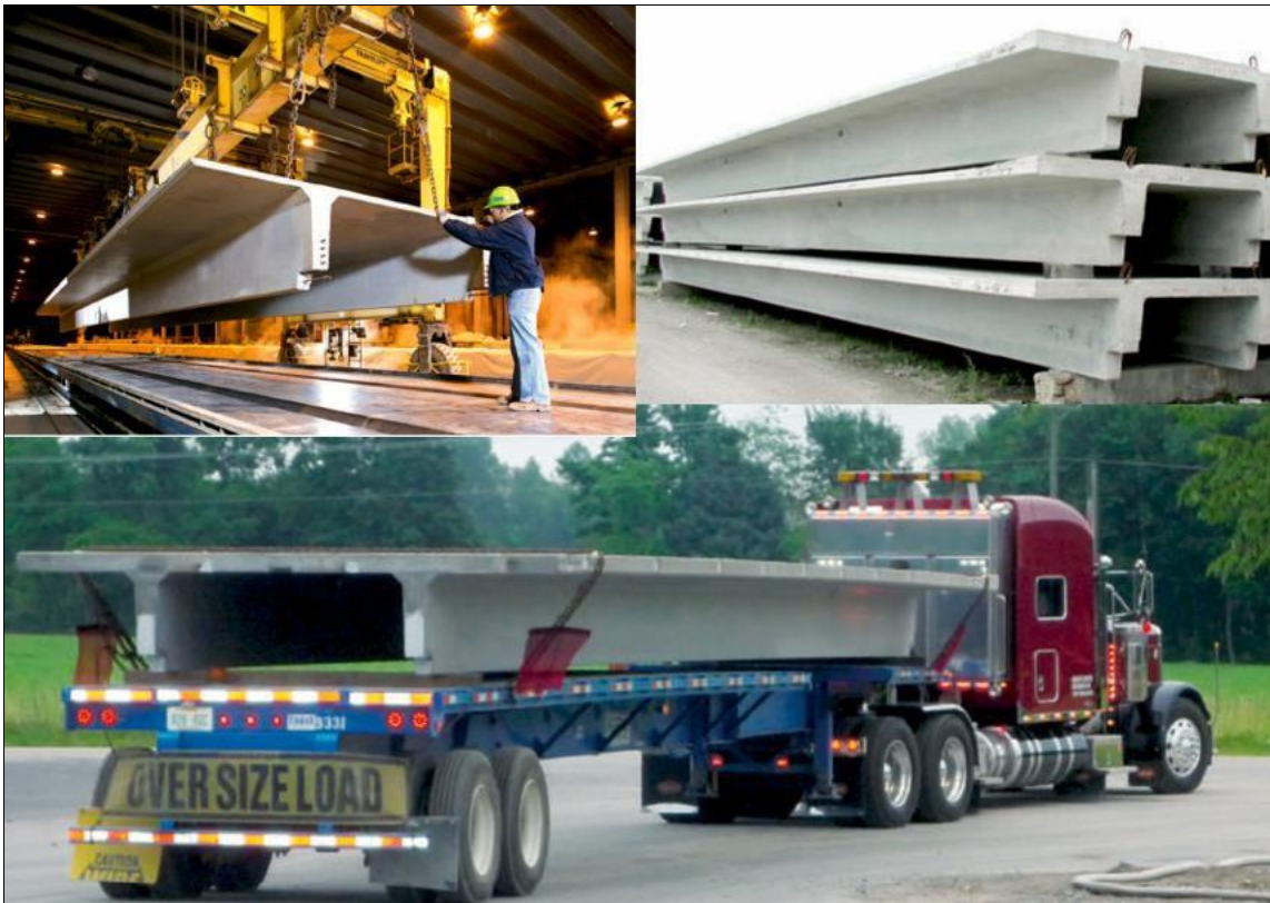
Figure 4 : DT member fabrication, stripping, storage and transport (PCI MNL-120-17)
