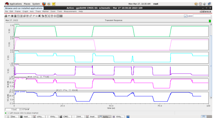
Fig -16: Peak-Power value and Total-Power value of CMOS 64-Bit graph
