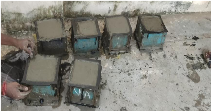
Fig 5: Casting the concrete
