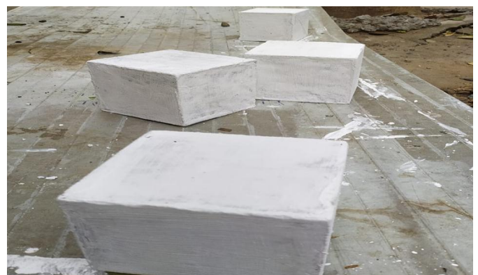
Fig 7: Applying of wax Curing of concrete cubes
