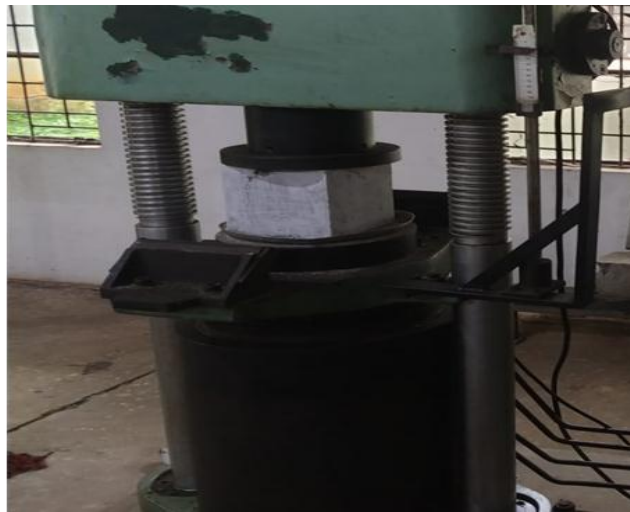
Fig 8: Compression test on cubes
