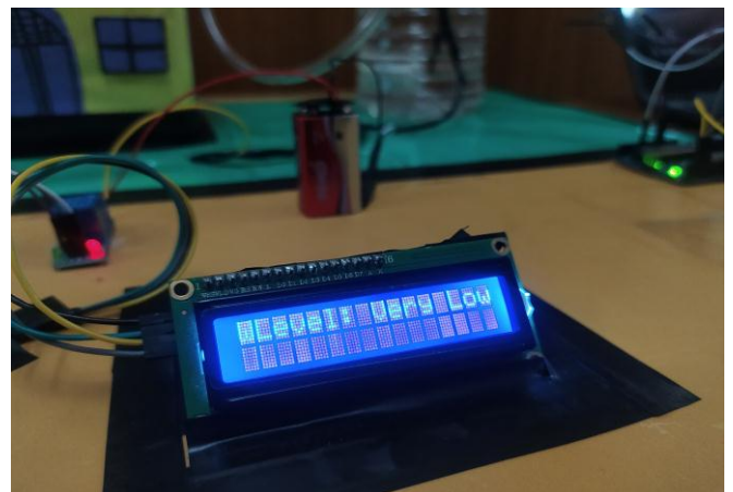
Fig.6: Water level status Low in LCD Display
